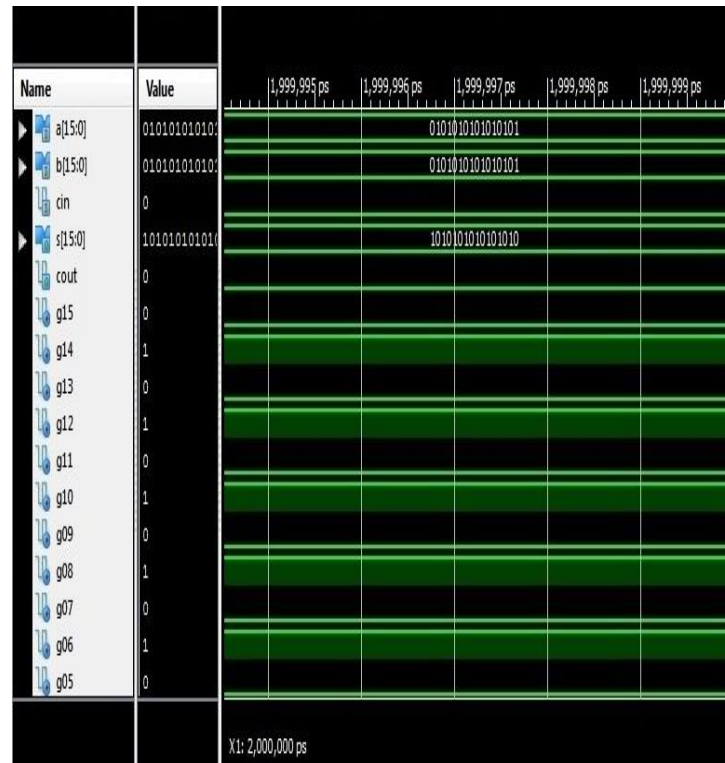
Fig. 4: Simulation Result of 16 bit Kogge Stone adder
