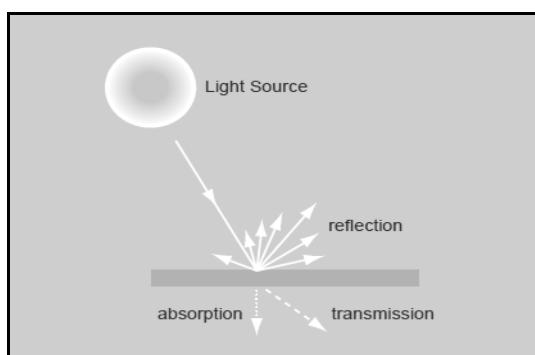
**Fig.1:** Process of reflectance.
