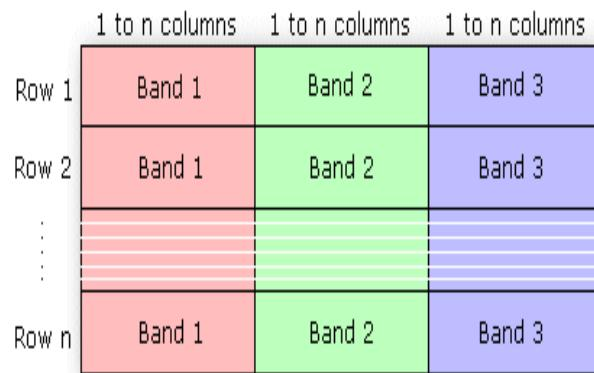
**Fig. 2:** General Structure of BIL Format.
