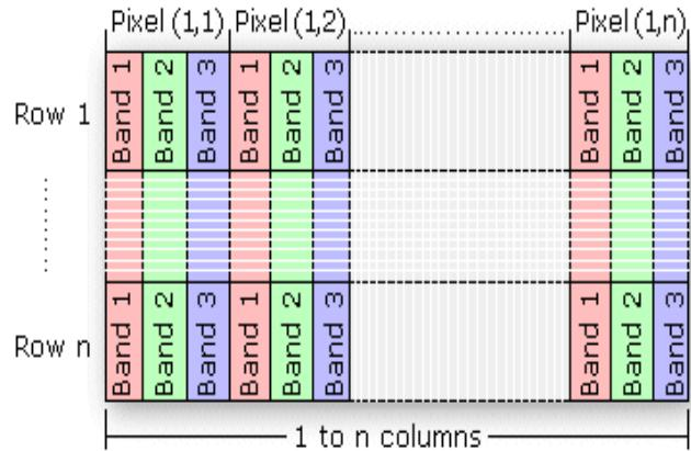
**Fig. 3:** General Structure of BIP Format.
