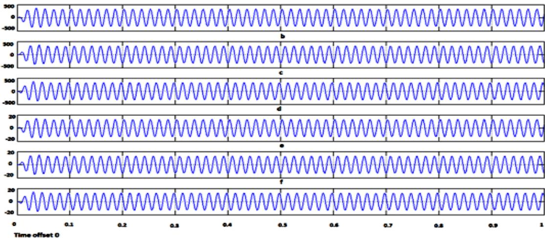
**Fig.6:** Line voltage and line current of Inverter with filter for PV stand alone system a.  $V_{ab}$  b.  $V_{bc}$  c.  $V_{ca}$  d.  $I_{ab}$  e.  $I_{bc}$  f.  $I_{ca}$
