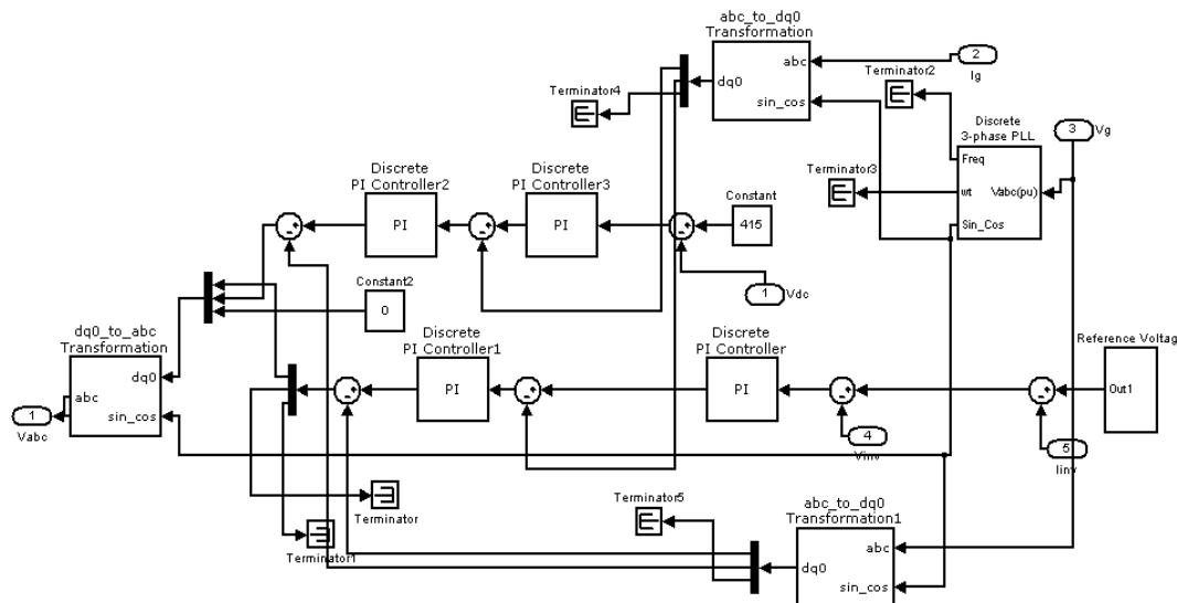
**Fig.3:** Simulation model of inverter controller for grid connected PV system
