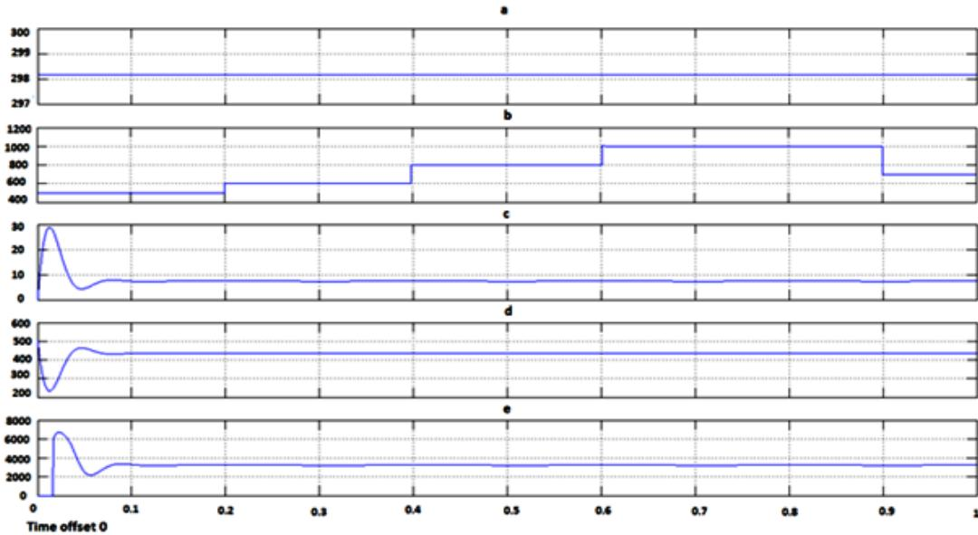
**Fig.4:** Boost Converter outputs connected to RLC Load through Inverter a. Temperature b. Solar Irradiation c. Current d. voltage e. power
