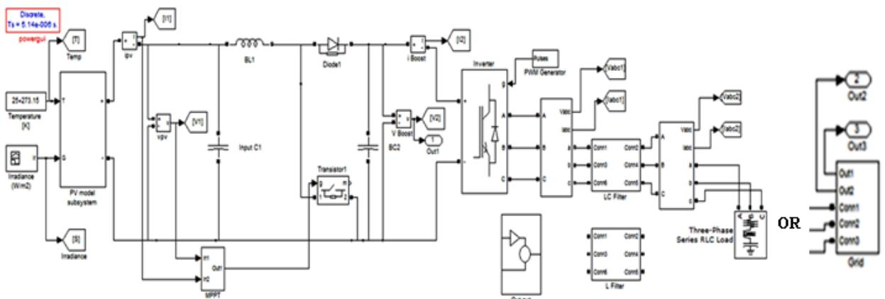
**Fig.2:** Simulation Model of Standalone or grid connected PV System
