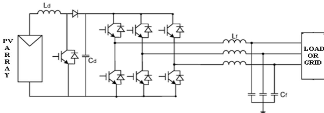
**Fig.1:** Stand alone or grid connected Solar PV system
