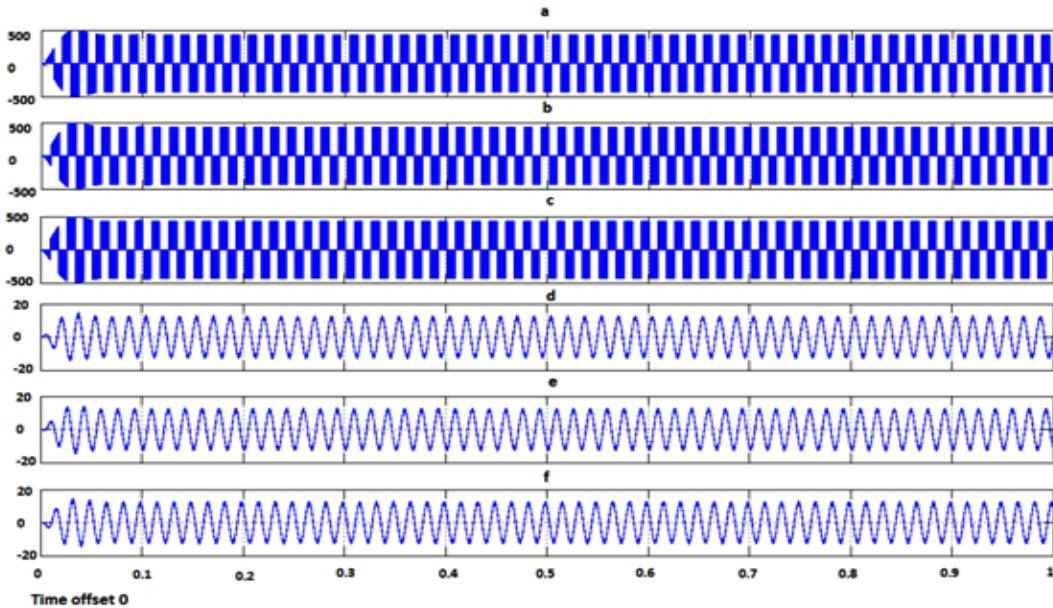
**Fig.5:** Line voltage and line current of Inverter without filter for standalone PV system a.  $V_{ab}$  b.  $V_{bc}$  c.  $V_{ca}$  d.  $I_{ab}$  e.  $I_{bc}$  f.  $I_{ca}$
