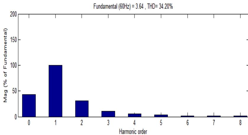
**Fig.9:** FFT analysis of Line Current with LC filter
