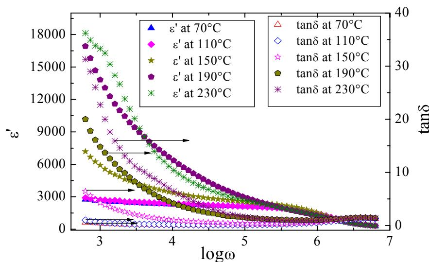
**Fig. 3:** frequency dependence of dielectric constant ( $\epsilon'$ ) and  $\tan\delta$  of BFN-BT ceramic at different temperatures.
