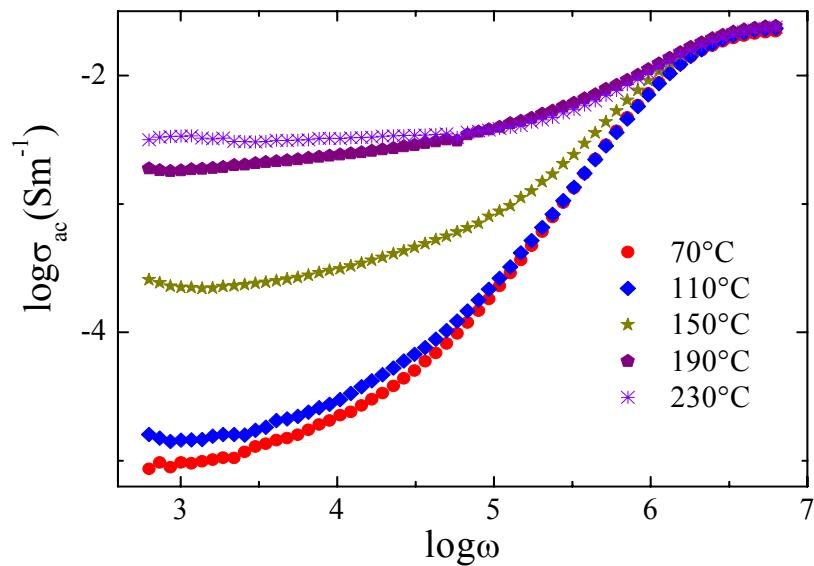
**Fig.4:** Frequency dependence of ac conductivity of BFN-BT ceramic at different temperatures.
