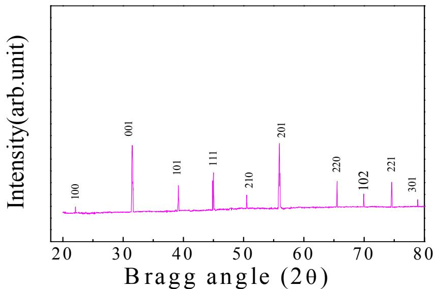
**Fig.1:**X-ray diffraction patterns of BFN-BT ceramics, at room temperature.
